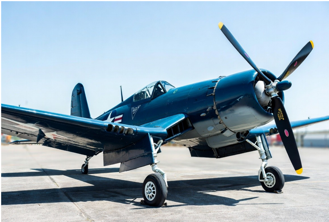
A Pratt & Whitney R-2800 Double Wasp radial powering the F4U produced 2,000 horsepower via three massive four-metre blades of Hamilton Standard Hydromatic constant-speed propeller.
